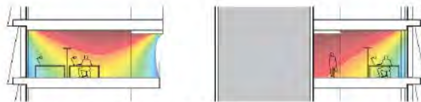
fig. 02. 3rd floor section with daylight factors
