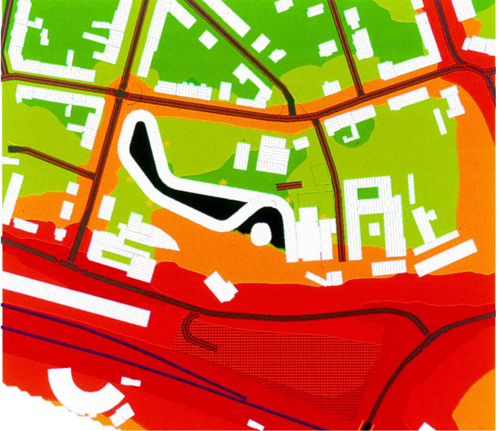
environmental agency dessau: diagram depicting the infiltration and intensity of noise sources near site (rail, street traffic, industry)
