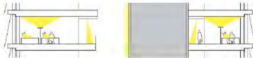
fig. 03. typical section; artificial lighting concept
