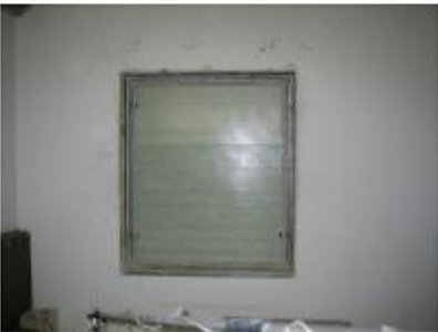
picture No. 3: GFK panel in test opening
