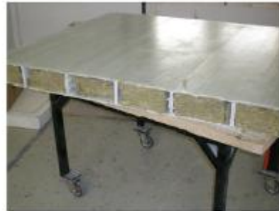
picture No. 2: GFK-panel with mineral wool filling
