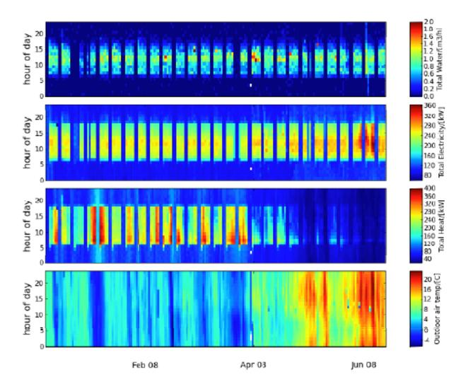
Carpet/raster plot: water, electric, heating load, outside air temp (BuildingEQ Project)
