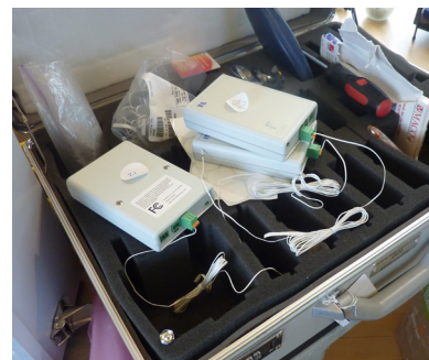
A large number of wireless sensor devices are part of CBE's field study toolkit.
