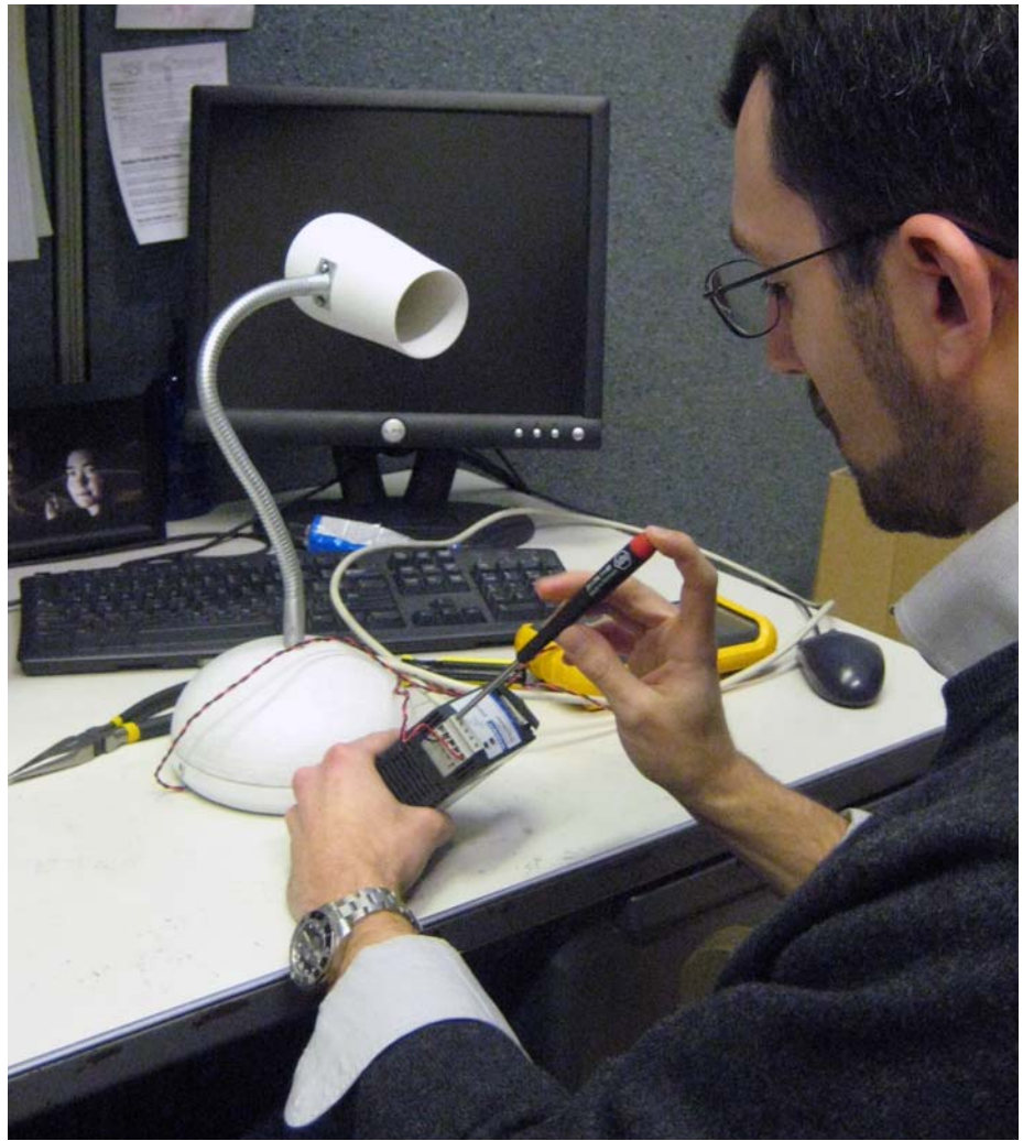
Graduate student researcher David Fannon works on the first generation prototype for the low-energy desktop fan.
