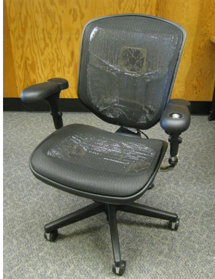
CBE's conditioned chair prototype incorporates reflective materials and low energy fans. Controls are located in the left arm rest.
