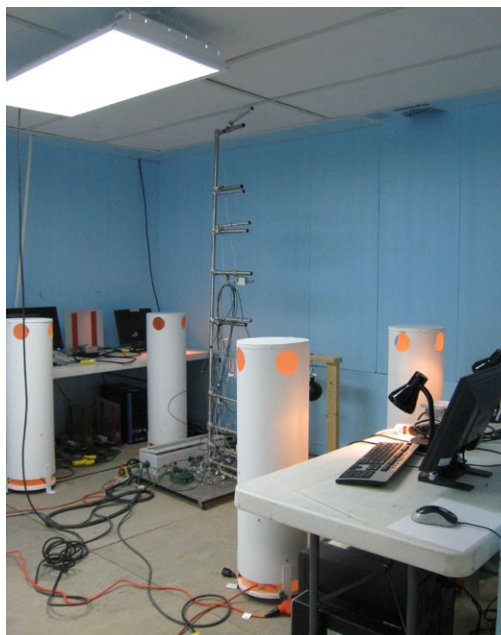
Test setup in Price Industries' test chamber showing simulated loads, sensor "tree" and radiantly cooled ceiling.
