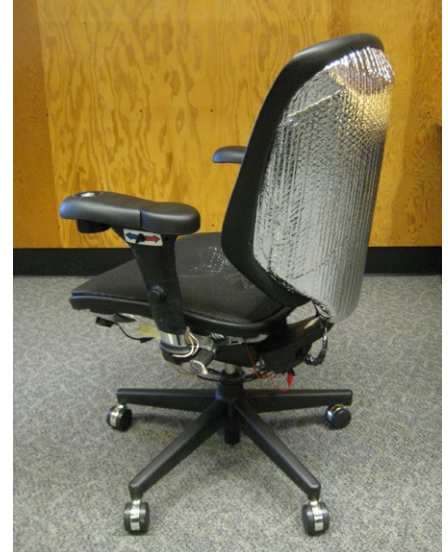
CBE's conditioned chair prototype incorporates reflective materials and low energy fans. Controls are located in the left arm rest.
