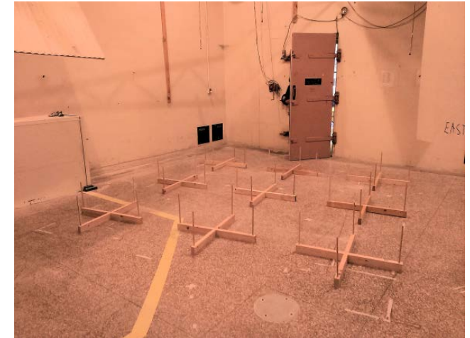
Reverberant room, NRC testing
