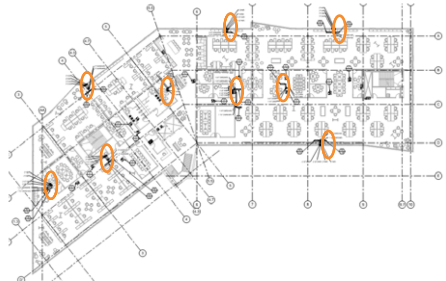
Multiple risers: Typical floor piping layout
