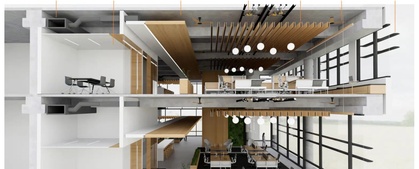
Clark Pacific's integration of ceiling fans into their radiant systems.
