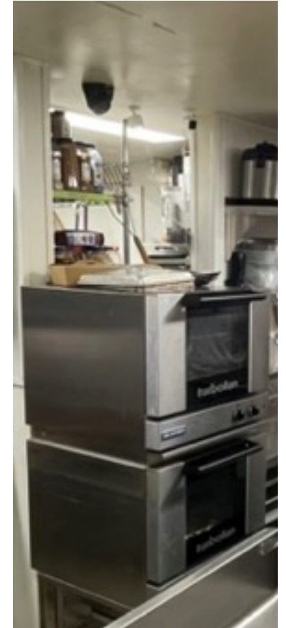
Unhooded double-stack convection ovens
